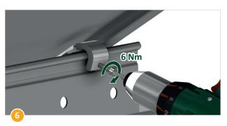
Tighten M6 bolt to 6 Nm +/- 0.5.
