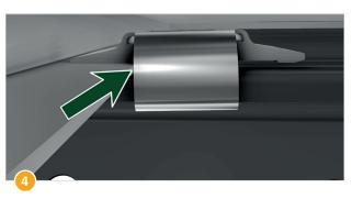
Clamping clasp must rest against module frame.
