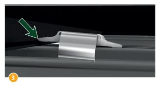
Lift the clamp slightly and push it over the module frame
