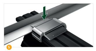
At least 1 grounding pin per module frame is required for grounding the array.
