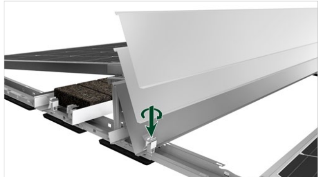
Fixate the Wind Deflector using the Universal Clamp.
