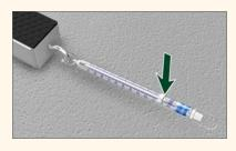
Before each measurement the scale has to be set to "O"
