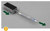
Pull the test weight with the spring tension scale transversely to the roof pitch.
