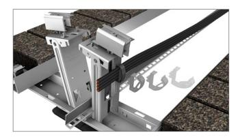
Press the Cable Clip into the recess provided on the Ridge Adaptor or on the Quarter-Point Strut. Insert the cables and close the Cable Clip.
