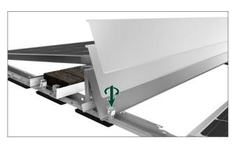
Hook the Wind Deflector into the Ridge Adaptor. Fasten the Wind Deflector with the Universal Clamp.
